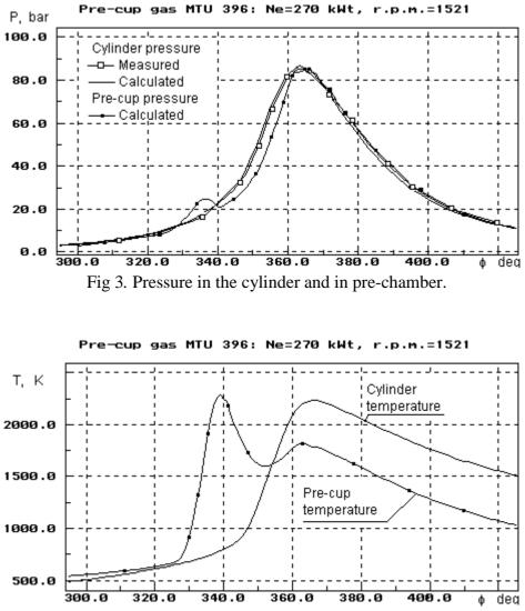
Fig 4. The in-cylinder average temperature and pre-chamber temperature.
