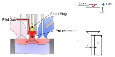
Fig 2. Scheme of pre-chamber.
