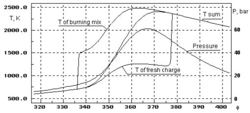
Fig 1. Curves of pressure and temperatures in the zones during combustion in SI petrol engine.
