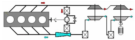
Boost : Two-stage electrically assisted turbocharger with total PR ~ 5.8
