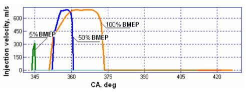
Injector design : should be matched with piston bowl and optimized together with parameters noted above.
